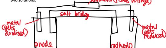
In one solution, substance is being oxidized, generating electrons. This side of the cell is called the "anode;" negative charge originates here. The other side of the cell receives the electrons, uses them for reduction reactions, and is called the "cathode."
