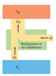
flow. Now, the heat going into the high temperature reservoir is the sum of the work and the heat that leaves the low temperature reservoir. To judge how well a heat pump works, we use the ratio of the heat that leaves the low temperature environment and the work put into the system. The objective is to get as much heat out and with the least amount of work put in.
