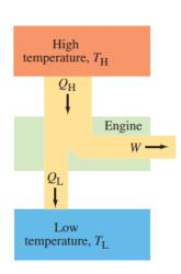
operating temperatures. Heat that flows out of the high temperature environment is equal to the sum of the work done and the heat going into the low temperature environment. Ideally, we would want to be able to use all the heat release for work, but this is not possible as a low temperature environment is necessary to cause heat flow. So we consider the efficiency of the engine, which is
