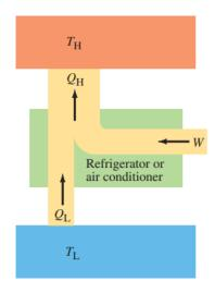
Now, the heat going into the high temperature reservoir is the sum of the work and the heat that leaves the low temperature reservoir. To judge how well a heat pump works, we use the ratio of the heat that leaves the low temperature environment and the work put into the system. The objective is to get as much heat out and with the least amount of work put in.
