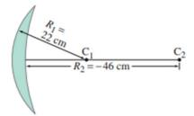
The converging surface (convex) is positive; the diverging surface (concave) is negative.
