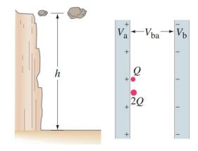
from the positive side to the negative side, the potential energy decreases. This electric field uses the potential energy to do work on the charge and push it to the negative plate.
