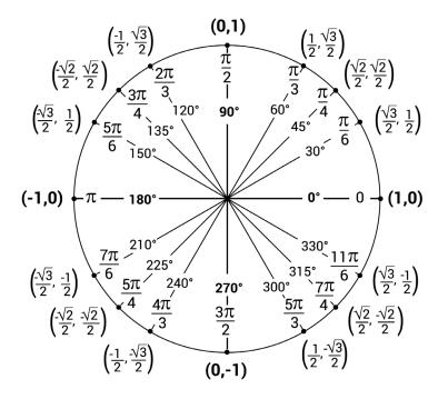
If we call one of these angles  $\theta$ , the point (x, y) at which the terminal ray of the angle intersects the unit circle is given by
